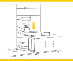
The  $d^2$  flexural modulus averages ±45 GPa for full section flexural testing, with some select profiles achieving over 65 GPa for a given span.
