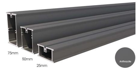
Available in three sizes (25mm, 50mm and 75mm), Dura Bearers can be installed directly onto hard surfaces, such as concrete or paving, as well as onto soft surfaces such as soil, sand or grass, (provided the area has been compacted and bricks, pavers or concrete slabs are placed beneath the bearers at suitable intervals).
